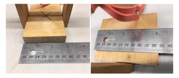
Cut two cup blocks at ¾ inch thick by 2 ¾ inch wide by 1 inch deep as pictured below.
