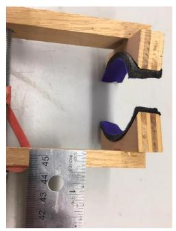
Drill a 3/16ths hole up 3 ½ inches in the middle of the staves as in the first picture. This is so later and when it is assembled a piece of all thread can go through both holes with a wingnut, washers and a locking nut. You will also need to install four small nails (two on each stave) as pictured above. The nails will be used to hook rubber bands onto the staves in the bending process.
