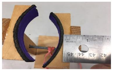
Cut a radius of 3 ½ inches into the cup blanks leaving ¼ inch in the middle of the radius and 1 inch at each end as pictured above.
